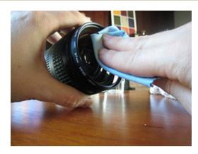
To clean my lenses, I will need my rocket blower, a clean micro fiber cloth and a dry washcloth. It's really important that you keep your micro fiber cloth in a separate case, because if dust gets on the cloth, you might end up grinding the dust into your lens. After blowing off the surface of the front and rear glass elements of the lens to get rid of dust or http://digitalphotographyblogs.com/2008/08/08/how-to-clean-your-camera/ (4 of 10) [4/12/2009 8:58:34 PM]
